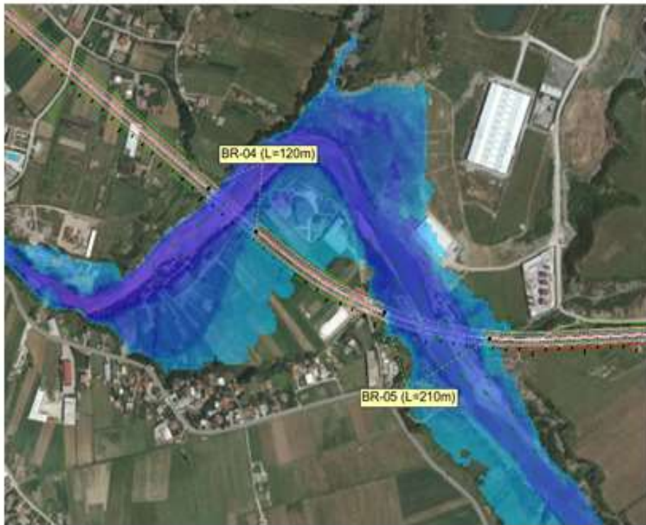
Figure 2.1 Hydraulic modelling of the four (4) Erzeni river bridges
